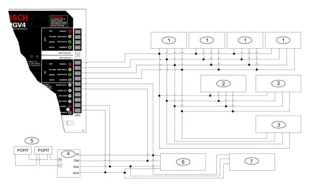
Figure 3.5: D7412GV4 SDI and Zonex Devices System Wiring Diagram
